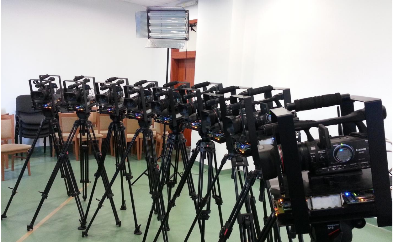
Figure 5. Multi-camera setup used in production of “Poznan Blocks” test sequence.
