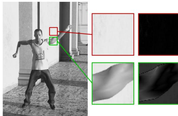
Figure 19: Mode preselection based on texture luma variance.
