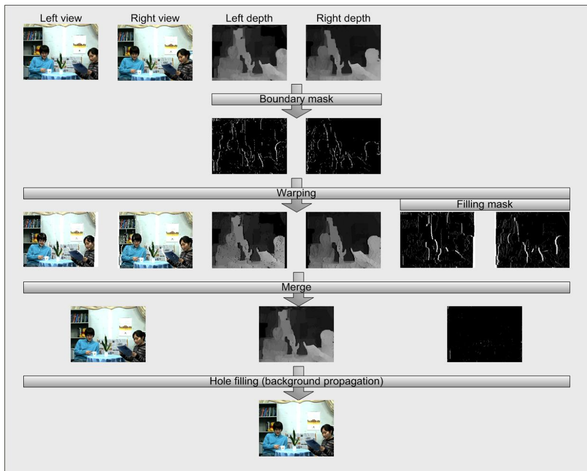
Figure 28: Flow diagram for VSRS 1D mode.
